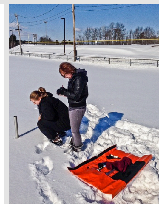
Figure 3. Collecting snow depth and density data in the field.
