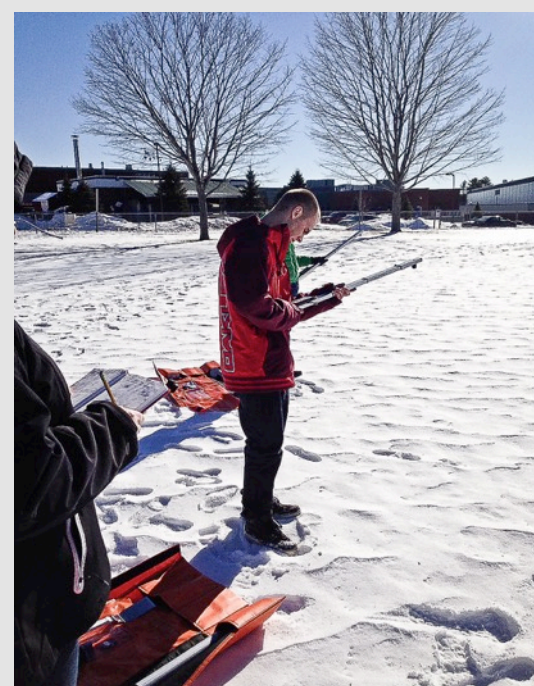
Figure 1. Measuring incoming and outgoing shortwave radiation using a pyranometer.
